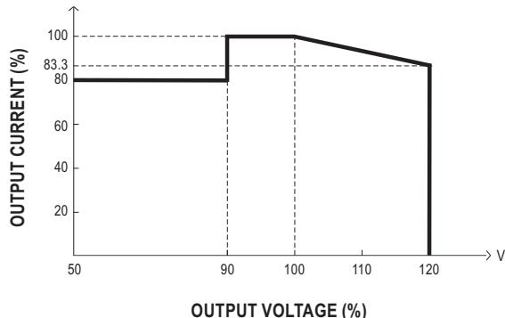
◎ The rated current should change with the Output Voltage Programming accordingly.
