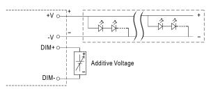
"DO NOT connect "DIM- to -V"
